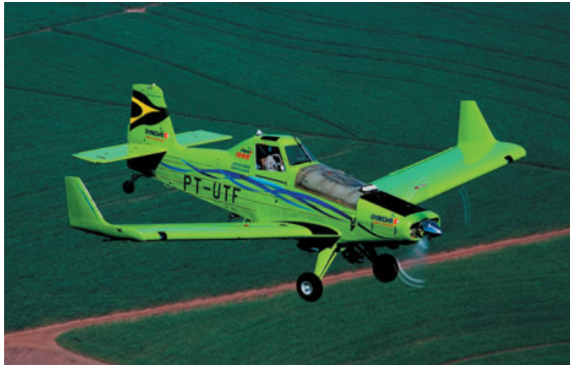
The Ipanema - the first ethanol-fueled production aircraft
